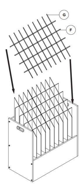
A. Place the assembled edge channel's on top of the built structure of the Horizontal Panels (F) and the Vertical Panels (G).
