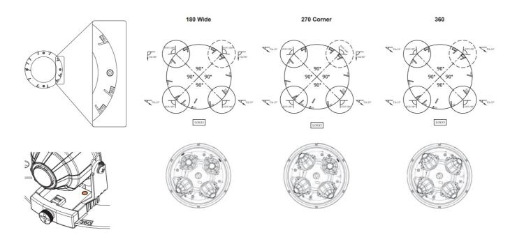
Adjust the main camera position to align it with the yellow dot indicated above on the chain ring (360-degree).
