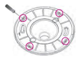
3. Use a driller to drill 4 holes in the surface where the positioning label is placed. Insert 4 screw anchors into the holes and secure the plate to the ceiling using the screws for the anchors.
