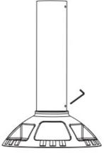
2. Choose a desired installation location and use a driller to drill 3 holes on the surface for securing the pendant
