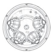
Adjust the main camera position to align it with the yellow dot indicated above on the chain ring (270 degrees).
