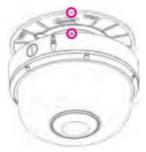
7. Twist the camera counterclockwise until it is secured firmly in place. Then fix the camera on the ceiling with the screw.
