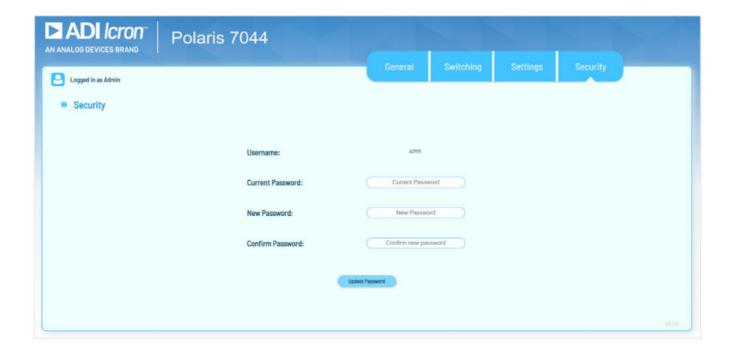
The security tab is used to manage the ADMIN and USER account access including changing the current logged in user.
