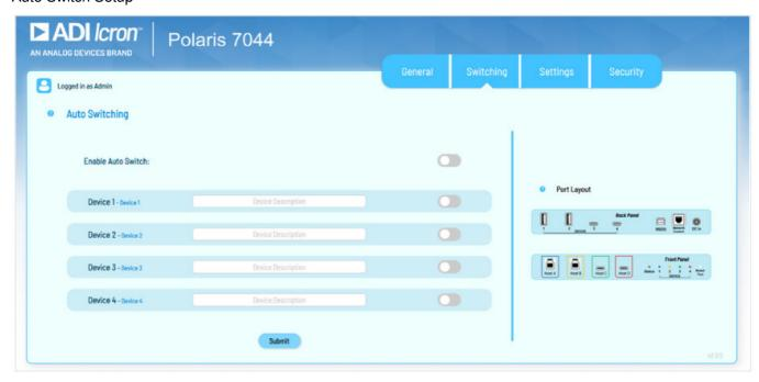
This tab specifies which downstream ports should auto switch to the most recent connection if the setting is enabled. At the top of the tab's context, a check box is used to enable/disable this feature. Below the check box, buttons are used to select downstream ports which should auto switch. Selected ports are highlighted. To apply changes to the Matrix, press the "Submit" button.
