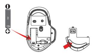
1. Remove the battery cover from the mouse and insert one AA battery and place the cover back on
