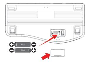
1. Remove the battery cover from the keyboard and insert two AAA batteries and place the cover back on
