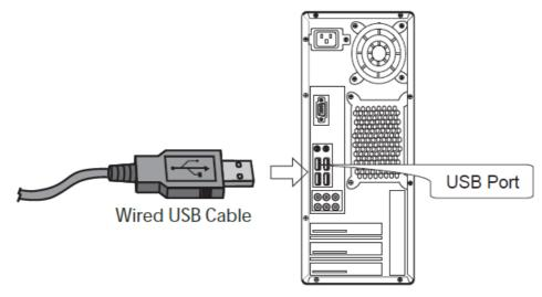
3. Turn On your computer; the operating system will detect the device automatically, no driver required.
