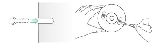
Use the drilling tool to punch holes on the wall according to the hole distance of the base. It is recommended to mark the holes on the wall with a pencil before drilling. Screw the expansion nut into the holes on the wall, and then connect the bracket to the expansion nut with screws to complete the fixing.
