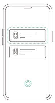
2. Enter the name and password of the Wi-Fi network you want the camera to connect to. To ensure long-distance connection, the camera only supports a 2.4GHz WiFi network with a stronger signal. Penetration capability does not support Wi-Fi with enterprise-level authentication. Please make sure that the Wi-Fi meets the requirements, click Next after completion, and the app can try to connect the camera to the Wi-Fi.
