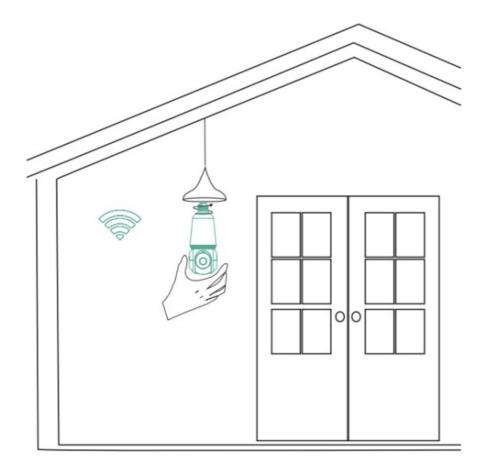
Please install the camera face down as shown in the picture. Wrong installation method may lead to product leakage and rapid damage
