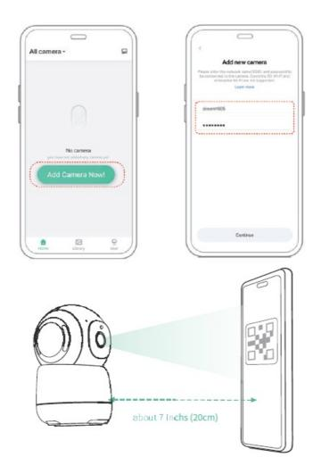
Click the "Add Device" in the App and enter the Wi-Fi network name and password that you want the camera to connect. Target the camera at the QR code of the mobile App, with a distance of about 20cm (about 7 inches) until the camera emits a "Di" sound, which represents the scanning is succeeded and the pairing is started.
