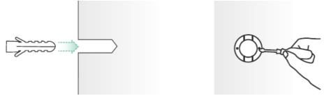
• Fix the camera to a desired location. You can directly place the camera on a flat surface, or fix the bracket to the wall or ceiling by screws, and then screw the camera to the fixed base.
