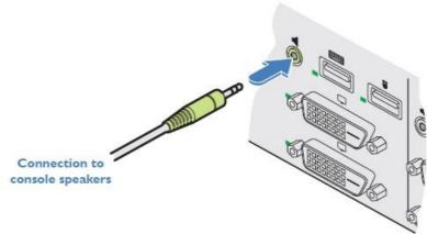
4. Insert the lead from the console speakers into the 3.5mm audio output socket on the rear panel.
