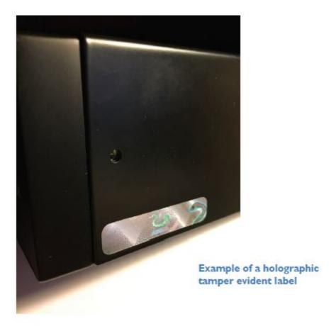
If for any reason one or more tamper-evident label is missing, appears disrupted, or looks different than the example shown here, please call Technical Support and avoid using that product.
