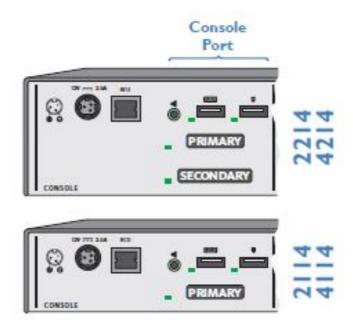
The video display(s), keyboard, mouse and speakers are attached to the various connectors on the rear panel that constitute the console port. Note: The secure switch can be used either with video display(s) connected to the console ports (KVM configuration) or alternatively with displays connected to each computer to allow the operator to view them all simultaneously (KM configuration) – see page 15.
