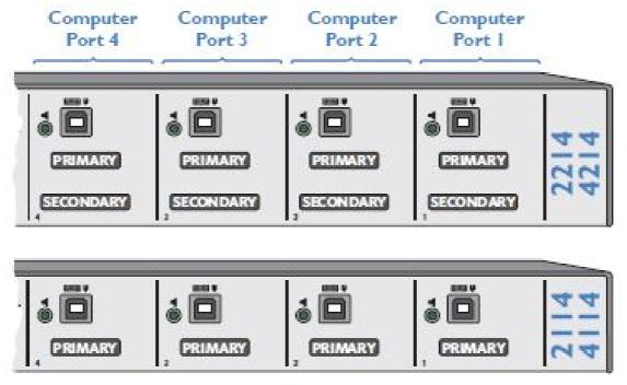
The green indicator associated with each console port should be ON to signify correct communications with the peripheral device. The video indicator will flash on power up whilst the switch is reading the EDID from the display. As a security measure, once the video indicator is ON the switch will not read the EDID again unless the switch is power cycled.
