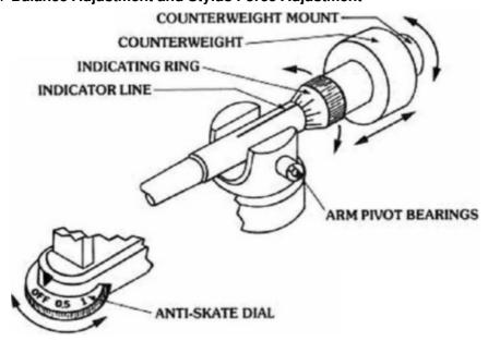
Turn the anti-skating dial to OFF as shown in **figure 7**. Remove a separate type stylus guard from the cartridge, or lift a flip-down type stylus guard while making your stylus force adjustment.
