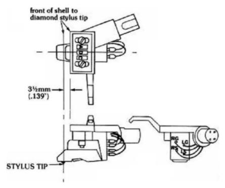
**See figure 4.** Hold the cartridge with its stylus tip approximately in the 32mm (.139") position shown and lightly tighten the cartridge mounting screws. Connect the lead wire terminal clips to the terminals of the cartridge with colors corresponding as follows:
