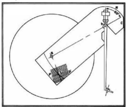
Place the TEMPLATE | hole 'B' over the spindle of your turntable, see figure 8.
