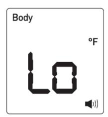
With the power on, press the Mode button to switch between body mode and surface mode. Body mode is used for measuring human body temperature. Surface mode is used to measure an object's surface temperature. (The factory default is "body" mode.)
