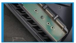
6. REMOVE THE SINGLE SCREW AND THE WASHER-LIKE STANDOFF UNDERNEATH.
