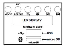
Below the LED display is a USB port for inserting a flash drive (USB pen drive) and below this is a slot for a micro SD card (or TF card)
