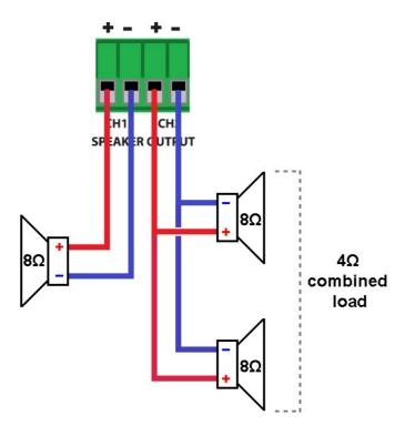
This means that if two  $8\Omega$  speakers are connected to a single output in parallel, they will each receive half of the full power. If the amplifier is delivering 50W to two  $8\Omega$  speakers connected in parallel, they must each be able to handle 25W.
