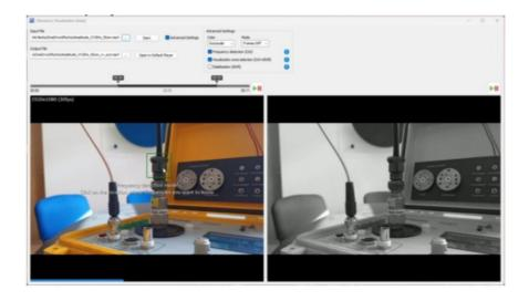
After processing, Detected Frequencies appear next to Advanced Settings. Main Freq. is found in the spectrum. Machine vibrations are often quicker than the usual video frame rate. Main Freq. may therefore be shown only due to aliasing. Actual vibration frequency may be a lot higher. It is listed below in a range of Possible Frequencies.
