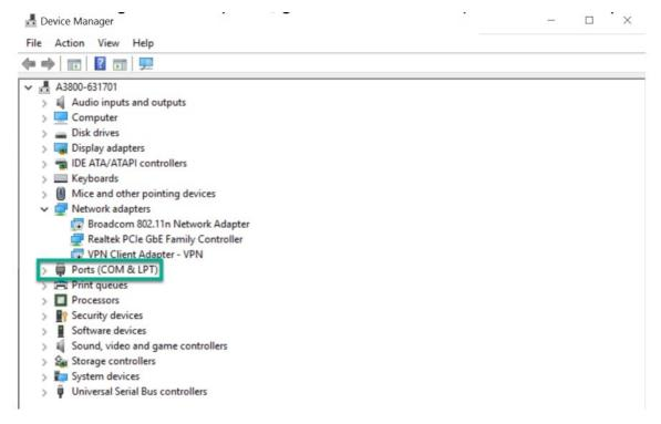
Find the port where your relay/loop module is connected (in our case it is port COM6). On which port your module is connected? Open Ports tab in device manager as shown in the following picture.
