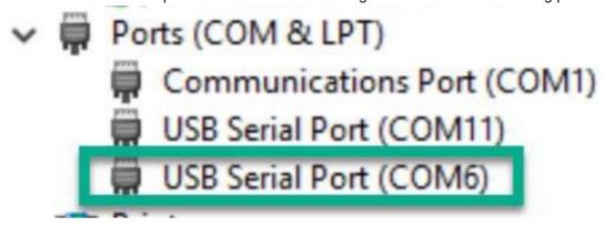
Then disconnect the module from online unit. You can see which COM port number is shown/hidden when you connect/disconnect your module.
