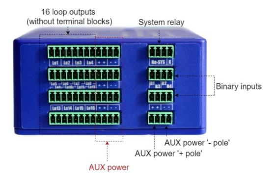
Terminal blocks are used to connect supply wire or to connect several wires together in electrical engineering. Where to connect these terminal blocks and how they look like is shown in the following picture. We connect terminal block for loop 1-4 and their powering.
