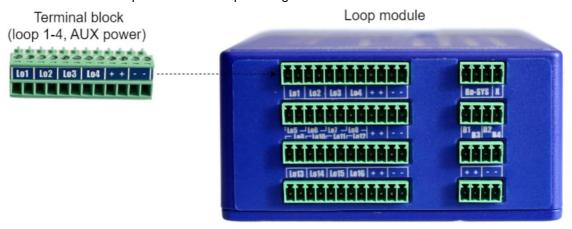
You can see top panel of loop module with terminal block connected in the following picture.
