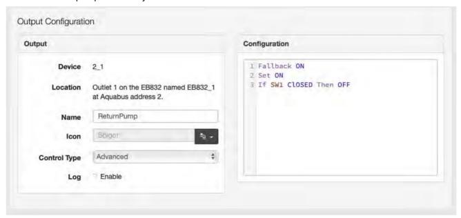
For example, when you want to do a water-change or there is an emergency such as water leaking/return blowing bubbles, the toggle switch can be activated to shut off the equipment.
