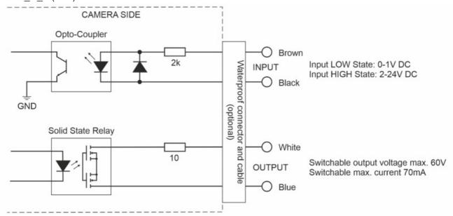
3.2.2. Einar camera connection diagram with IO cable and ParkIT junction box:
