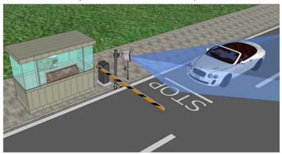
Try to adjust the direction of the camera so that the number plates are horizontal in the picture! From the point of ANPR/LPR the most important is the size of the characters on the image. It is recommended to have at least 25 pixel average character height. The too large characters are also not suitable for ANPR, therefore try to avoid settings where the character size is greater than 50 pixels in height.
