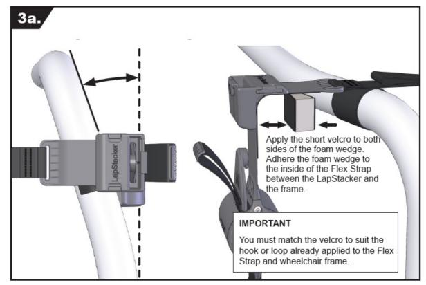
4. Attach LapStacker assembly to the frame.
