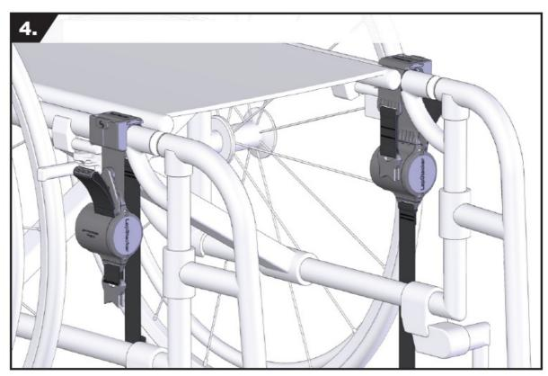
5. Pass Tension Strap around the lower tube, join buckles and tighten.
