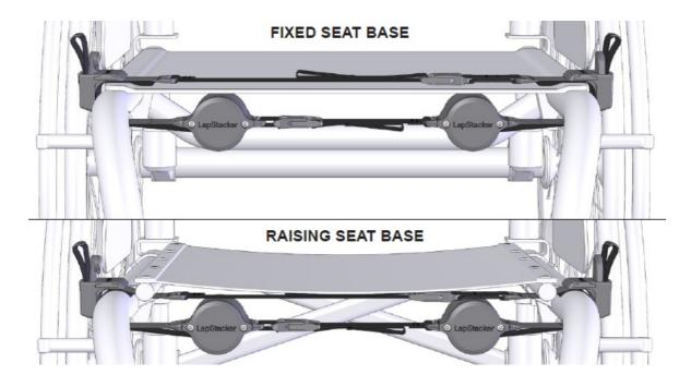
If you have a raising seat base, the LapStacker must pass under the seat base. Adapt install steps to suit.
