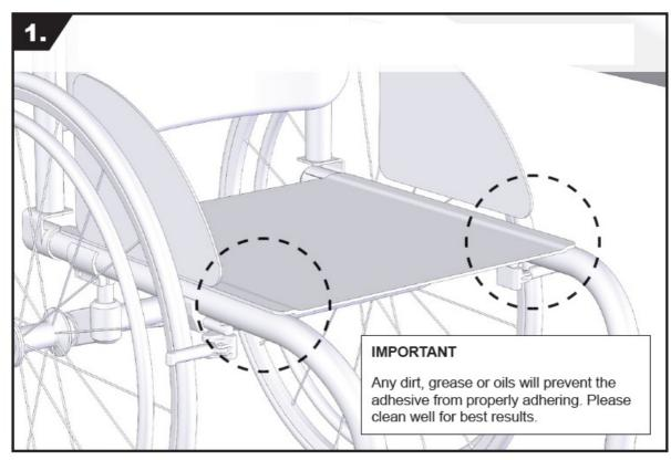
2. Adhere velcro to the frame and seat base where the Flex Straps will make contact. Repeat on each side.
