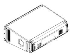
The CS10 is a sub-compact, powered, intelligent, line array enclosure designed for extended throw applications. It contains two symmetrically arrayed 10" LF transducers, and a 4" HF compression driver mounted onto an Adamson waveguide. The high frequency waveguide is designed to couple multiple cabinets across the entire intended frequency band without loss of coherence.
