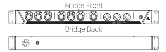
**Network Distribution System NDS (905-0039)** – The NDS is a network and analog path that allows users to send redundant audio and control to CS-Series loudspeakers on a single network cable. The NDS combines LAN A and B network ports using two external AVB enabled switches.
