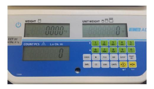
The scales have three digital display windows. These are "Weight", "Unit Weight" and "Count pcs". It has 6-digit display to indicate the weight on the scale.
