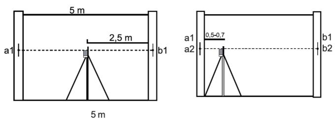
Choose a wall and set laser 5M away from the wall. Turn on the laser and the cross laser line is marked A on the wall. Find another point M on the horizontal line, the distance is around 2.5m. Swivel the laser, and another cross point of cross laser line is marked B. Please note the distance of B to A should be 5m. Measure the distance between M to cross laser lune, if the difference is over 3mm, the laser is out of calibration, please contact with seller to calibrate the laser.
