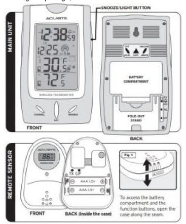
Acu-Rite instruments have been designed and engineered to provide accurate and reliable Measurements. Please read the instructions thoroughly before setting up your wireless thermometer. The remote sensor is designed to stand or hang. For wall mounting, use the enclosed screw to mount to the desired surface. Use the slot on the back of the case to mount the remote sensor to the surface.
