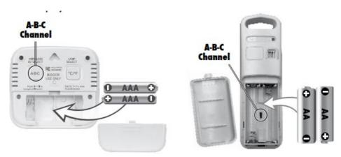
**NOTE:** If pairing more than one wireless sensor (model 06002 or 06044) with the display, the A-B-C channel must differ between each sensor. Verify that each sensor has a different channel selected by following the instructions in the corresponding sensor manual.
