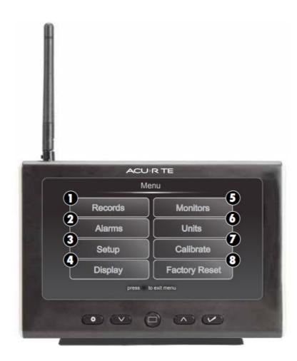
Navigate to the main menu at any time by pressing the " \*\* button. From the main menu, you can view records, set alarms, set up additional monitors, and more.
