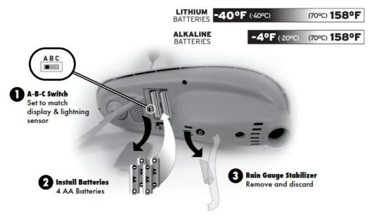
**NOTE:** If add-on sensors are being used with the display (see page 17), set them up at this time. If pairing more than one wireless sensor with the display, the A-B-C channel must differ between each add-on sensor. The display will automatically begin searching for add-on sensors during initial setup.
