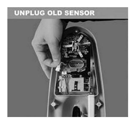
4.eUnplug the old temperature and humidity sensor by grasping the base of its white plug and gently removing it.
