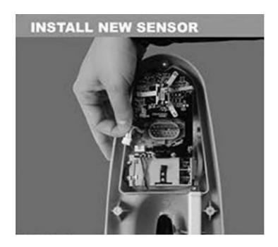
6.eSlide the new temperature and humidity sensor into place. Holding the base of its whittle plug, gently plug it into the connector.
