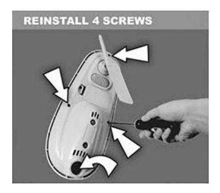
2.eRemove all 4 outer screws and separate the upper and lower portions of the sensor Set aside the upper portion and s crews for reassemble.
