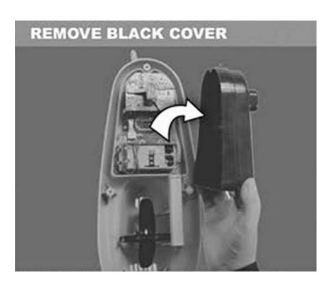
3. Carefully remove the black cover, setting it aside for assembly later.
