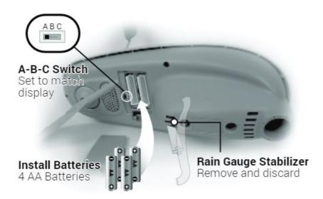
NOTE: In the battery compartment of the sensor, there is a small A-B-C switch that must match the selection on the display. By default, both the sensor and display are set to "A" and should not need adjustment.
