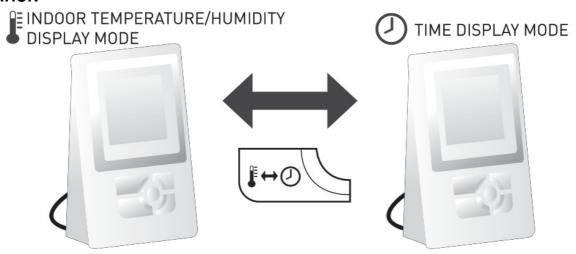
You may switch between viewing the current time or the indoor temperature by pressing the "Indoor Temperature/Clock Selection" Button.
