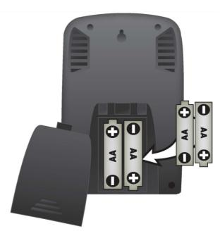
Slide the battery compartment cover open and install 1 fresh "AA" battery as shown here.
