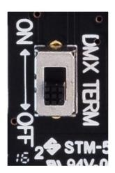
prevent signal reflection. If there is no connection to the DMX THRU terminals, the DMX Terminate switch should be ON.
