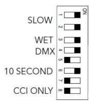
Note: Black is where the DIP switch position should be. On is to the right.
