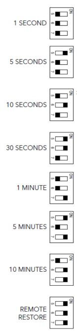
Example DIP switch setup for slow DMX speed, wet contact, 10 second restore time, and CCI only to trigger Emergency mode.
