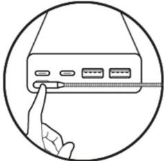
Connect the power cable, from the bottom of the Skinetic board, to the output USB C port of the battery. **Step 2**
