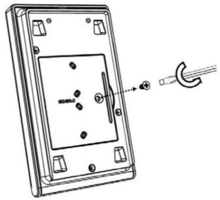
With a screwdriver, remove the screw holding the battery cover
