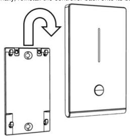
Remove the sensor from the mounting bracket by sliding the control upwards
