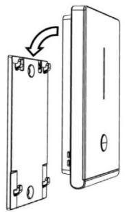
Slide the zone sensor downward onto the bracket
