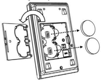
Once the cover has been removed you will have access to the batteries for replacement. Please note the battery type is CR2450
