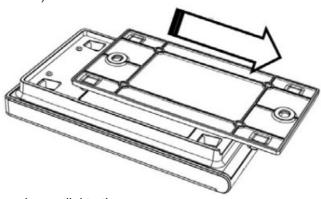
Slide the mounting bracket down, in parallel to the zone sensor
