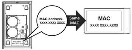
There is a MAC address on the back of the zone sensor. Check if the MAC address shown on the Touch controller matches the MAC address printed on the zone sensor.
