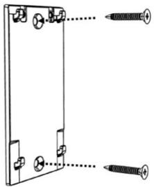
Fasten the mounting bracket to the wall using fasteners or double sided tape.
