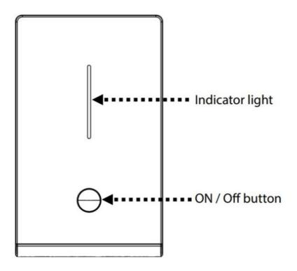
Indicator light (Blue): Pairing mode Indicator light (Red): Damper close Indicator light (Green): Damper open On/Off button: Open/close damper
