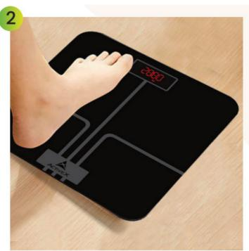
Step 2: Activate the weighing scale by pressing it gently either with your hand or feet. a
