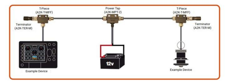
All NMEA 2000 networks require a 12V DC supply. In addition, a correctly functioning network will require the following components as a minimum:
