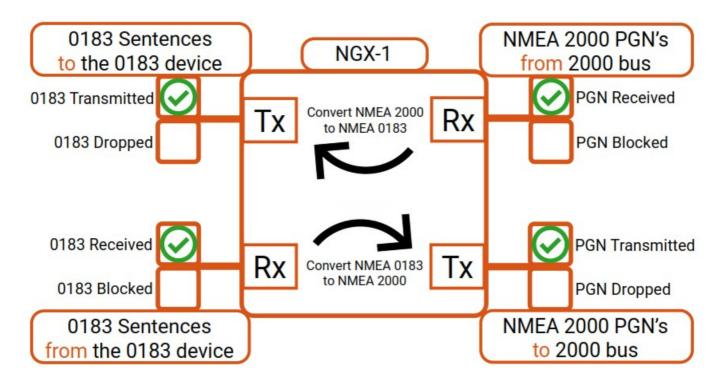
For a successful conversion to take place, you need to make sure that the required NMEA 0183 sentence to be converted is not only checked on the NMEA 0183 side to receive(Rx), but also that the corresponding PGN message is ticked for transmission onto the NMEA 2000 bus(Tx). A PGN cannot be transmitted onto the NMEA 2000 bus if it has not first been received from the 0183 device. The same convention applies for conversions from NMEA 2000 to NMEA 0183.
