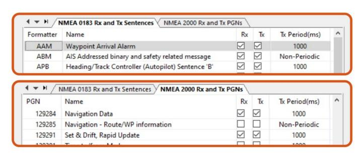
The NGX-1 offers the user considerable flexibility over what data will be converted, allowing messages to be blocked if not required, and also control over the transmit frequency (Tx period(ms)).
