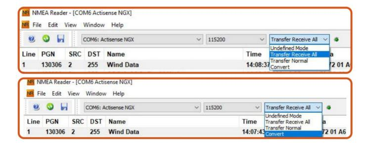
In addition to a change of Mode, the baud rate may also require alteration. This can achieved using the instructions overleaf.
