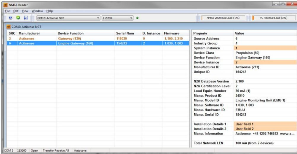
NMEA Reader is used to view all the NMEA 2000 messages on an NMEA 2000 network. This feature will be integrated in to Toolkit in a future update. If the same NGT-1/NGX-1 is to be used for viewing data in NMEA Reader as well as using Toolkit, the COM port in Toolkit will need to be closed (set to 'Offline') before it can be opened in NMEA Reader.
