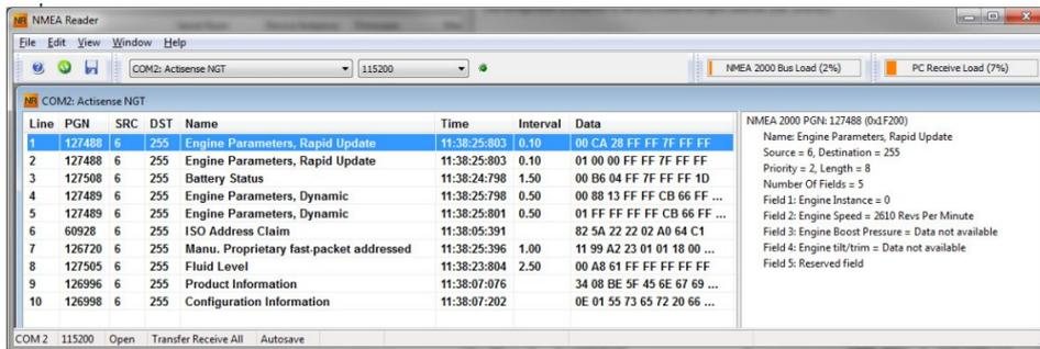
The EMU-1 on Source Address (SRC) 6 is also sending an Engine Parameters, Rapid Update PGN 127488 for the Starboard Engine (Engine instance = 1) that indicates its Tach input 2 is measuring the Starboard Engine running at a speed of 2612 RPM:
