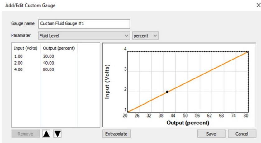
To be turned into a graph with a value for 0% to 100% output, where the EMU-1 then has a reference for voltages from 0-5V in this example:
