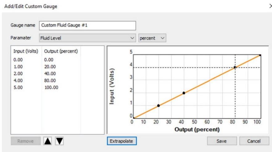
It is important to remember that the more readings that are added, the more accurate the custom gauge is going to be.
