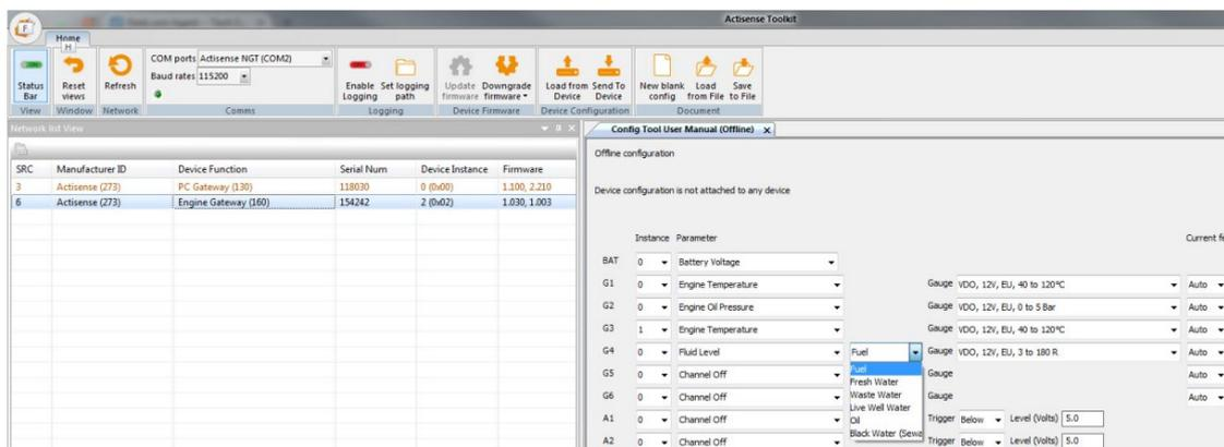
The default trigger level is 5 volts but that can be configured to any value which falls within the Alarm input range (of 0.1 – 40.0 volts).
