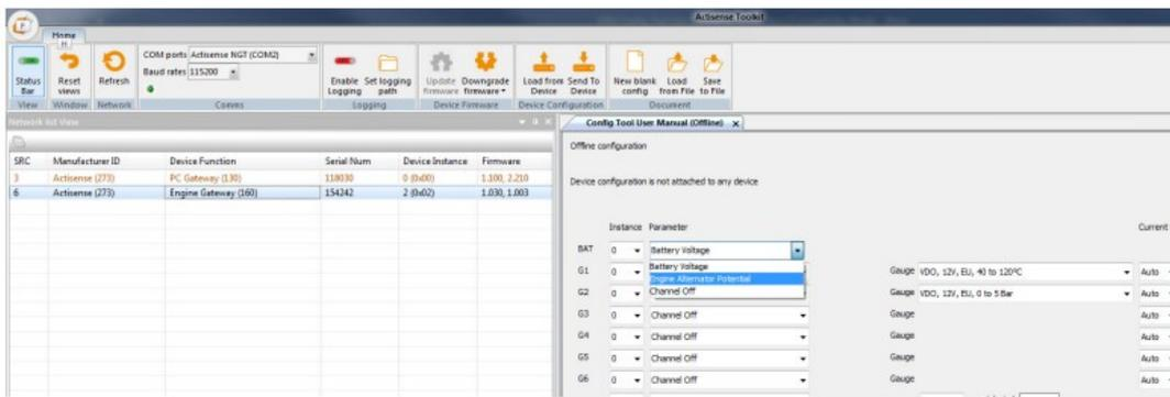
The BAT Instance selection becomes the Battery Instance in the Battery Voltage PGN (127508) or the Engine Instance in the Engine Alternator Potential PGN (127489). When Engine Alternator Potential is chosen, use Engine Instance 0 for the Port engine and 1 for the next engine (e.g. Starboard):
