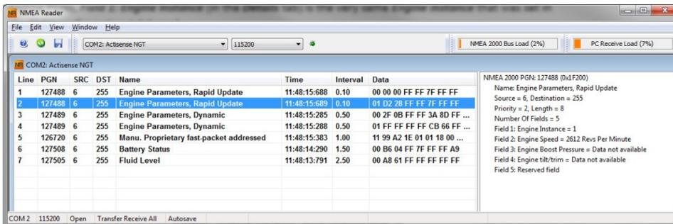
The EMU-1 on Source Address (SRC) 6 is also outputting Engine Parameters, Dynamic PGN 127489 and Fluid Level PGN 127505 as shown below:
