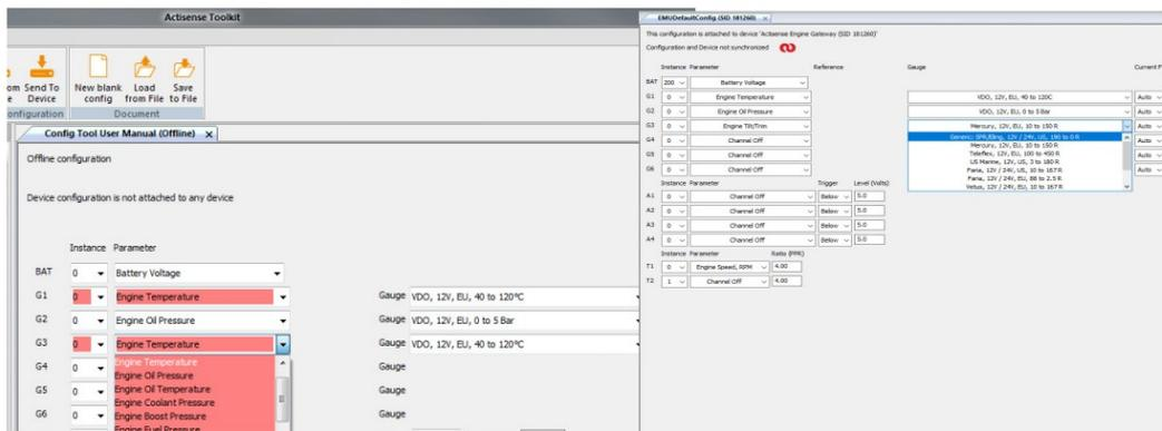
**Note:** Selecting a particular gauge assumes that the correct corresponding sender is connected to that gauge, hence selecting a gauge is essentially selecting the gauge / sender combination.
