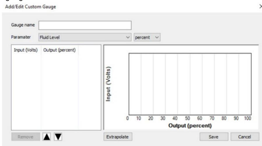
In this Window, the values are entered into the table on the left to start building the graph.
