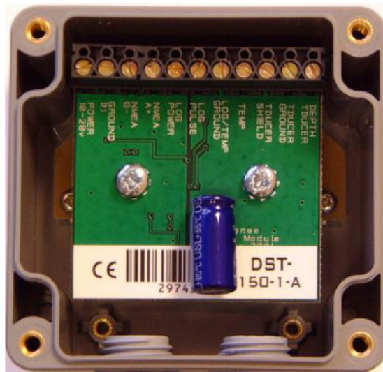
Figure 1 – View of the inside of the unit, showing external connections
