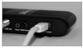
3. Plug the other end of the Ethernet Cable into an OPEN Ethernet Port on your Modem/ Router.
