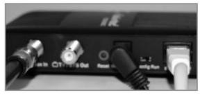
6. If necessary, get a second MoCA Network Adapter. Plug one end of the 2nd Ethernet Cable into the Ethernet Network port on the side of the 2nd MoCA Network Adapter.
