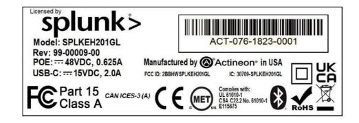
The above image represents an example of the serial number / regulatory marking label attached to each Edge Hub unit. Information regarding the regulatory standards with which the Edge Hub complies and the relevant markings included on the label are explained below.
