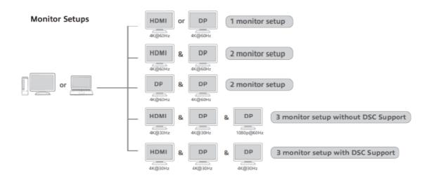
Your USB-C device needs to support DP-Alternate mode or Thunderbolt<sup>™</sup>3 on its USB-C port in order to display your video output to 1 or more displays. Check the technical specifications of your USB-C device if it supports DP-Alternate mode or Thunderbolt<sup>™</sup>3. If the device does not support DP-Alternate mode or Thunderbolt<sup>™</sup>3, the AC7046 will not be able to display video onto your Display(s).
