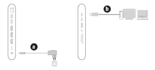
• a: Connect the plug of the power supply to the DC connector of the docking station and then connect the other end of the power supply into the wall outlet.
