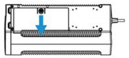
2. LIFT the battery out of the compartment, and disconnect wires from battery positive (+) and negative (-) terminals. Get a new battery and make sure to re-connect wires to positive and negative terminals correctly.
