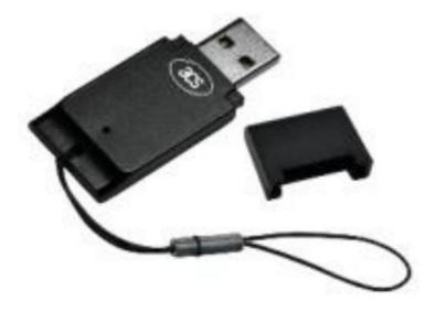
The ACR39T-A1 has PC/SC and CCID compliance, making it easy to install and use as it is specifically designed to be integrated into any computer-based environment. Its drivers are compatible with operating systems such as Windows , Linux , Mac OS and Solaris. In addition, the ACR39T-A1 may now be used with mobile devices running the
