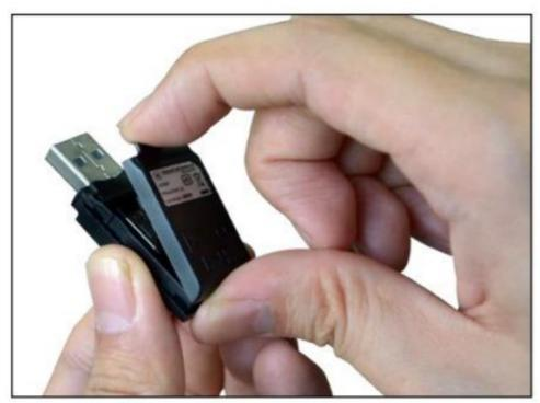
Remove the cover completely to insert/remove the SIM card to/from the reader.
