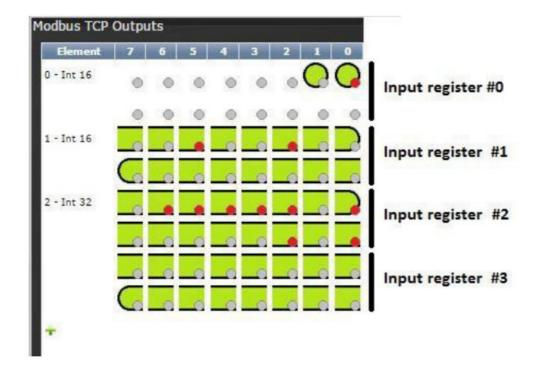
The controller's outputs can also be addressed as coils. The assigned outputs start at coil #16. The controllers outputs can be read with function code 2 "Read Input Status."
