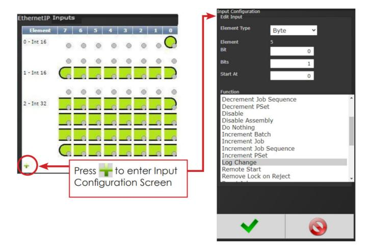
Example of the Ethernet IP Input screen with five Inputs set up.
