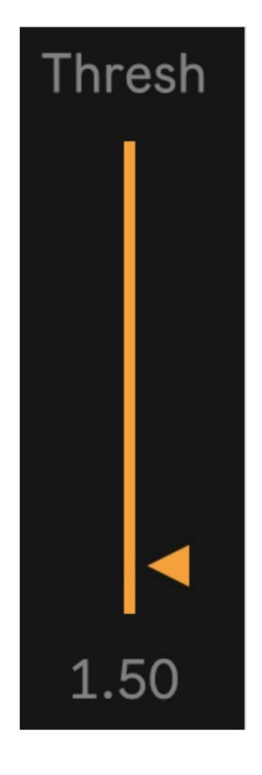
Setting the threshold high will cause quiet notes to be ignored, allowing the user to only trigger the device when they choose to play a note loudly. This allows you to trigger the device organically through expressive playing on your instrument.
