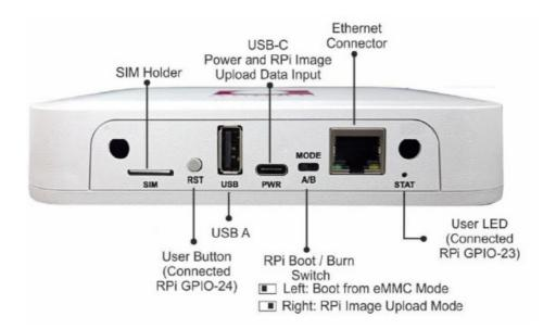
All the peripherals of the device are shown above. The Device comes with an Ethernet cable and a USB -C Power Adapter that is required to establish the remote connection.
