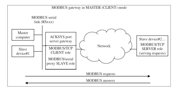
The Master on the serial line doesn't know the network address of the slave devices that it interrogates: those are identified on the serial side by an unique MODBUS address. A translation table in the administration menu establishes the correspondence between the MODBUS serial addresses and the corresponding IP addresses.
