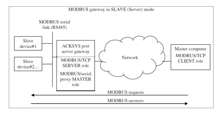
The port server gateway converts and transfers requests from the TCP clients towards the serial line, then wait for an answer and sends it back to the client. As the serial line may support several bussed slave Modbus peripherals, these ones are distinguished on the serial link by their own unique Modbus address. Therefore, on TCP side, the client application identifies each serial peripheral by its Modbus address and the IP address of the port server gateway.
