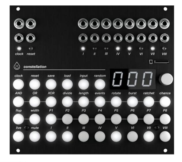
Constellation requires a +12V / -12v power supply with a 2×5 pin ribbon cable (included). The red line of the ribbon cable must be aligned with the -12V marking next to the module's power header and on your case's power distribution board. Constellation draws 75mA from the +12 rail and 18mA from the -12 rail. Please ensure you have enough power available before installing.
