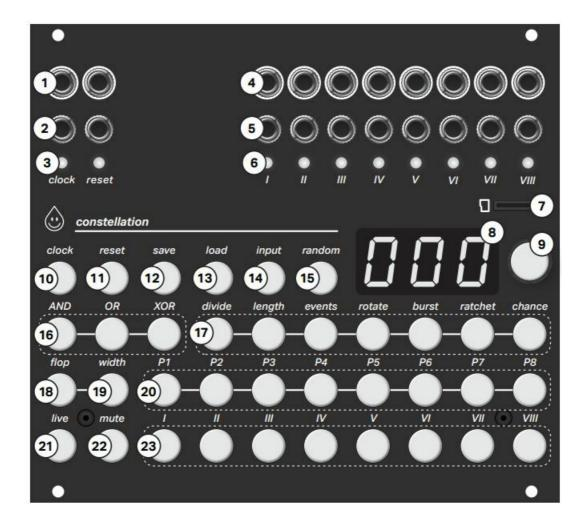
Constellation is comprised of 8 identical channels, each with a selection button (23), output jack (4) and output state LED (6). Within each of these channels, you can combine up to 8 unique looping patterns of different length and density to generate complex rhythmic output. Each pattern has a selection button (20) and a set of parameters selectable on buttons (17) and editable with the encoder (9) and numeric display (8).
