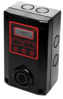
To calibrate the oxygen sensors, you would need a calibration gas that has a known concentration value, 100% nitrogen, a 0.5 LPM regulator, a calibration adapter, and tubing (see list of part numbers and linkson next page). We recommend calibrating the oxygen sensor every 3 months. You will need a cylinder of 100% Nitrogen(Zero Gas) and a cylinder of 20.9% Air(Span Gas).
