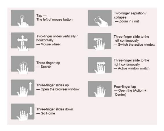
Touch pad function description (Android), must be switched to the Android system
